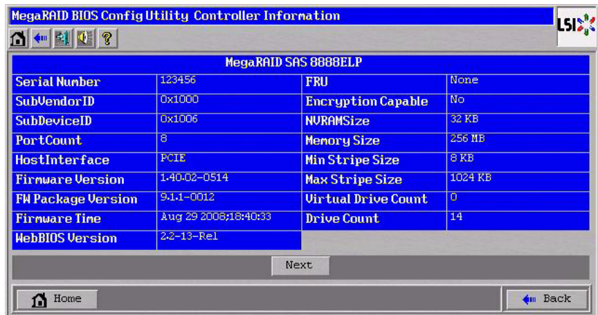
Figure 6.1 First Controller Properties Screen
